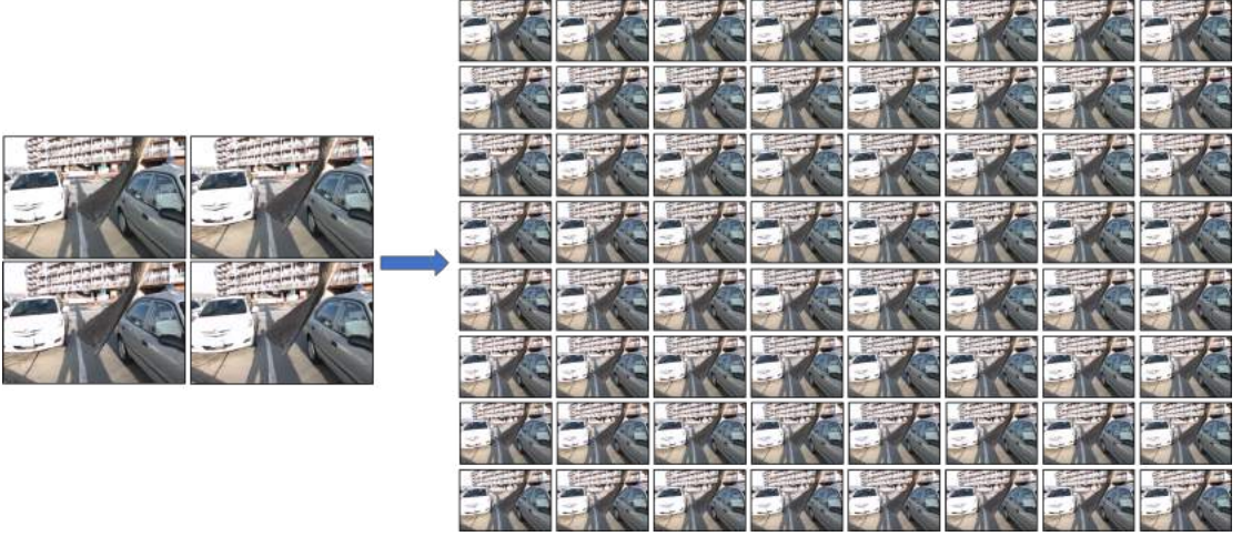
Figure 1.1: Using only four corner sub-aperture images of a light field with angular resolution 8 \times 8 , all other views of the light field are synthesized by our proposed approach.
