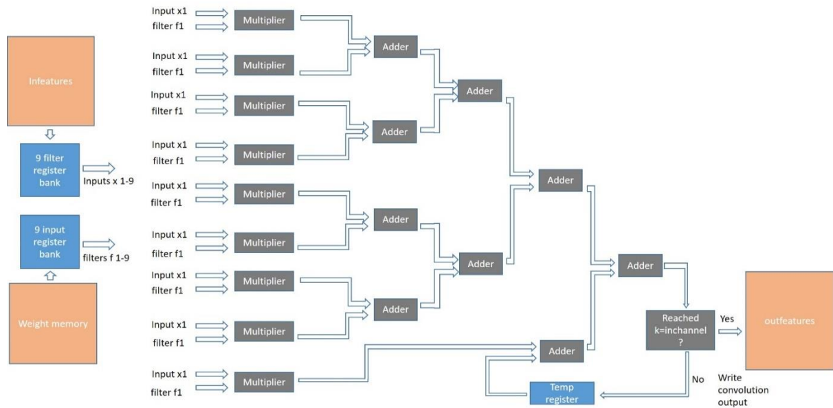
Figure 51 A Non systolic architecture for convolution
