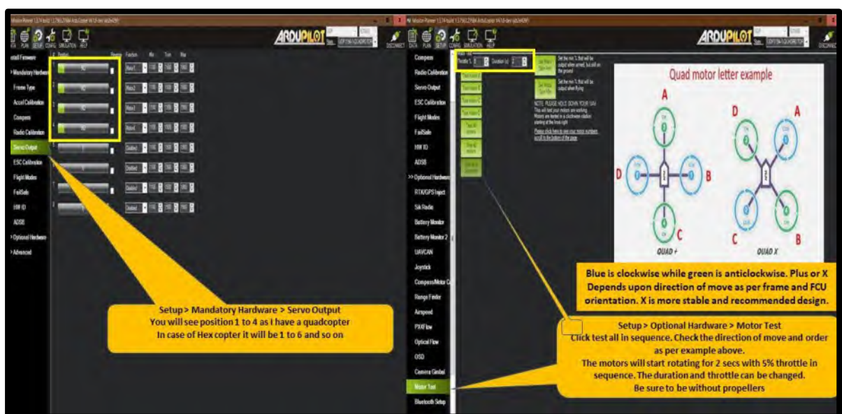
Figure 10.8: Checking motor/ESC detection and servo output and rotation direction including sequence
