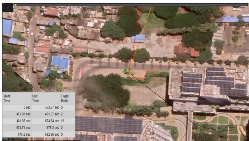
Figure 6.3: Hexacopter in Position Hold mode
