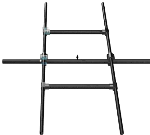
Figure 3.6: CAD Model: Pipe body frame
