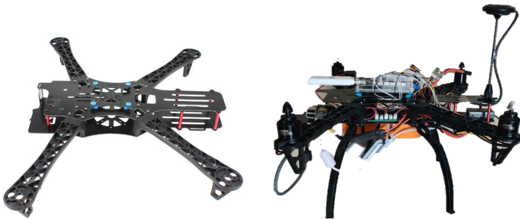
Figure 3.4: V-Type frame configuration
