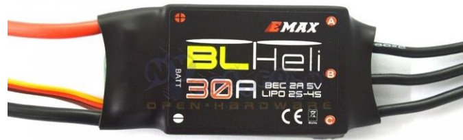
Figure 5.3: ESC with rating 5V 30A
