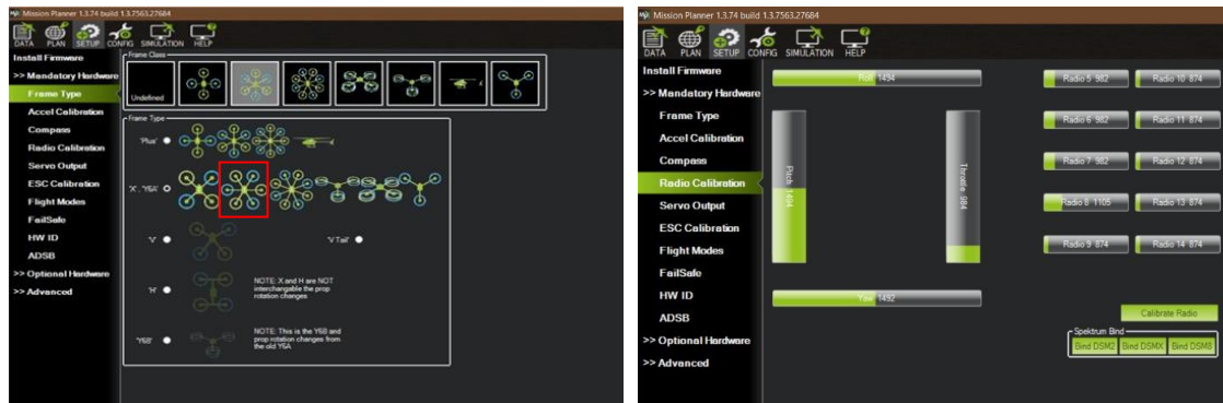
Figure 6.2: Mission Planner: a) Firmware selection b) Drone Calibration
