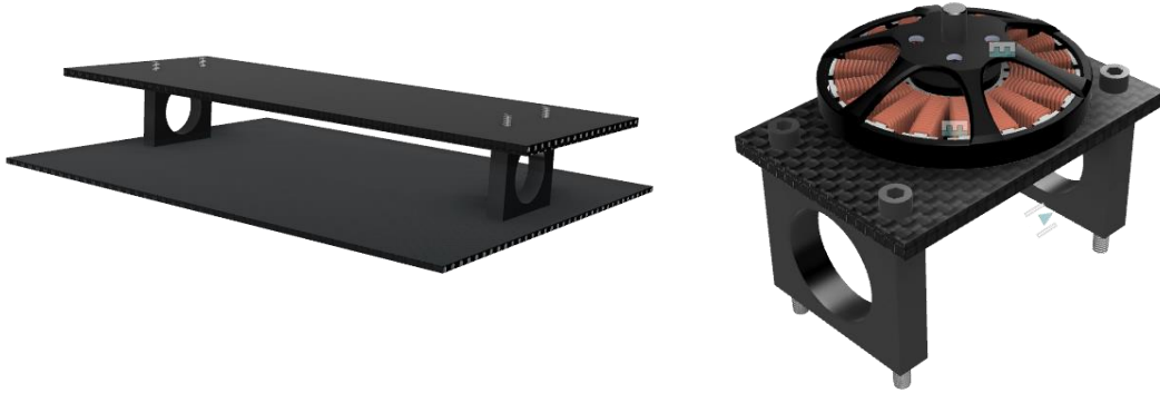
Figure 3.5: CAD Models a) Centre plate assembly b) Motor assembly
