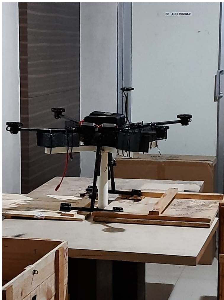
Figure 3.8: Table top testing of hexacopter X Frame for alignment
