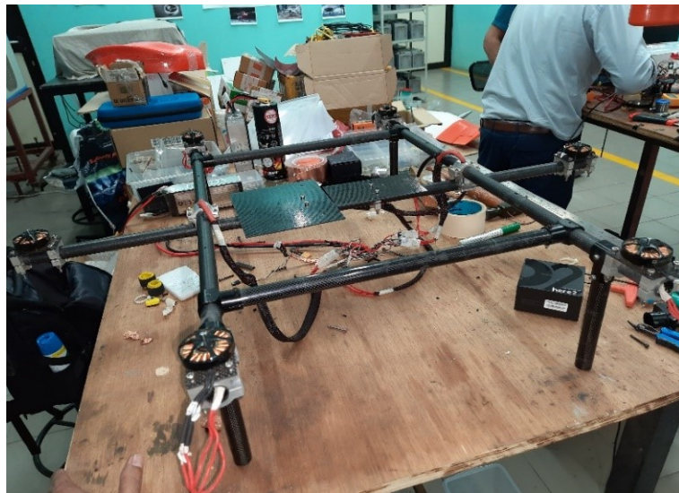
Figure 3.7: Assembling Hexacopter Drone Frame
