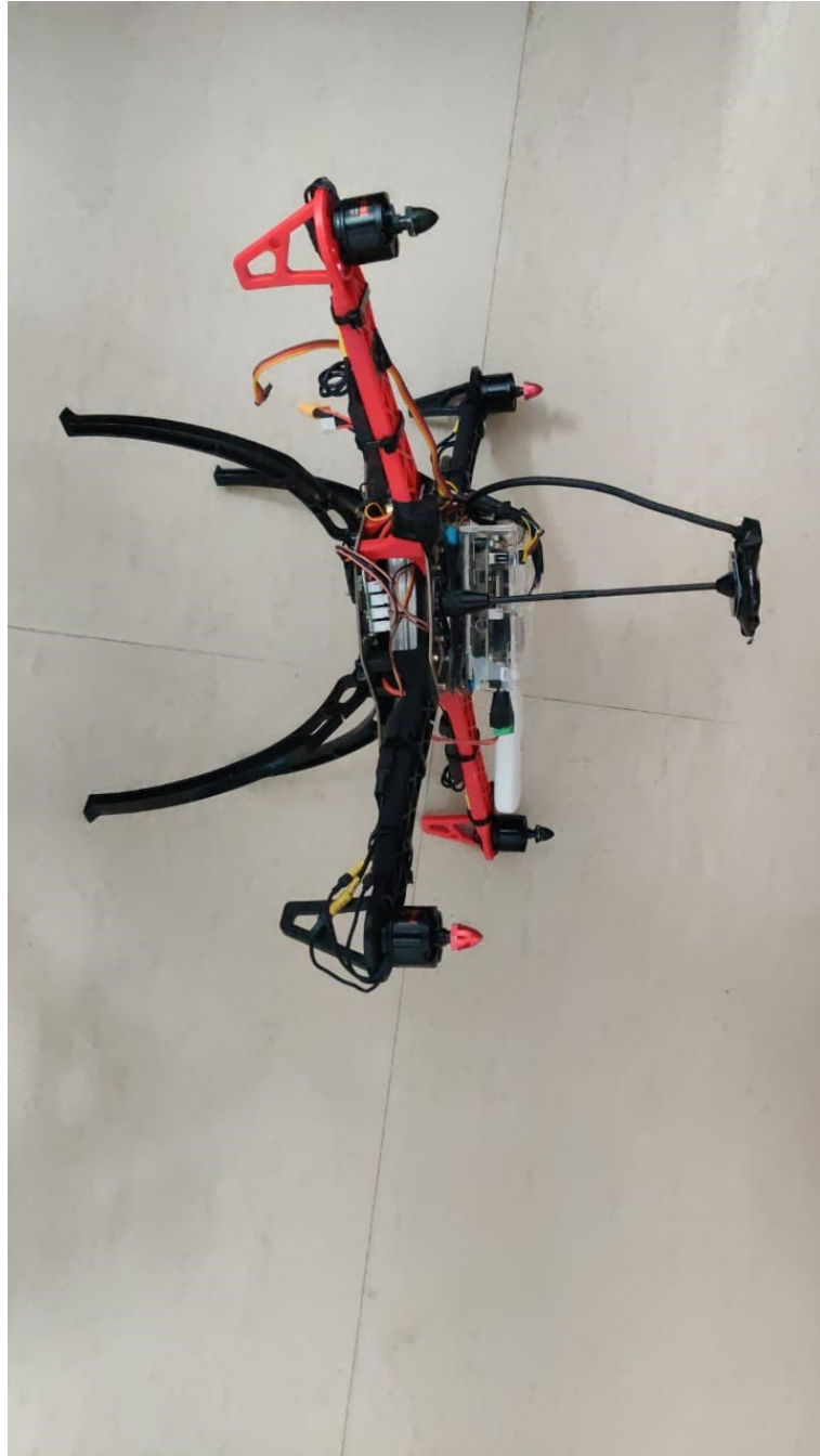
Figure 3.5: X Type frame configuration
