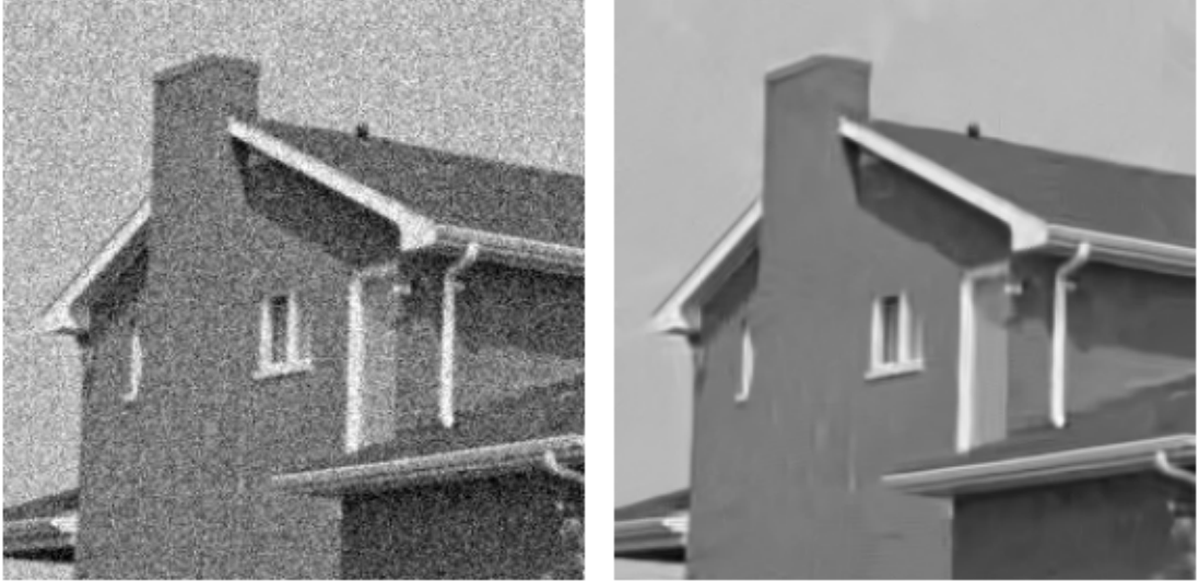
Figure 2.2: A sample result from BM3D. The image on the left is the noisy image ( \sigma = 25 ) and the one on the right is the denoised image. Image taken from Dabov et al. (2007) .
