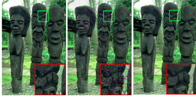
Figure 2.3: A sample result from DnCNN. The image on the left is the original image. The one in the middle is a noisy image ( \sigma = 35 ) and the image on the right is the denoised image. Image taken from Zhang et al. (2017) .
