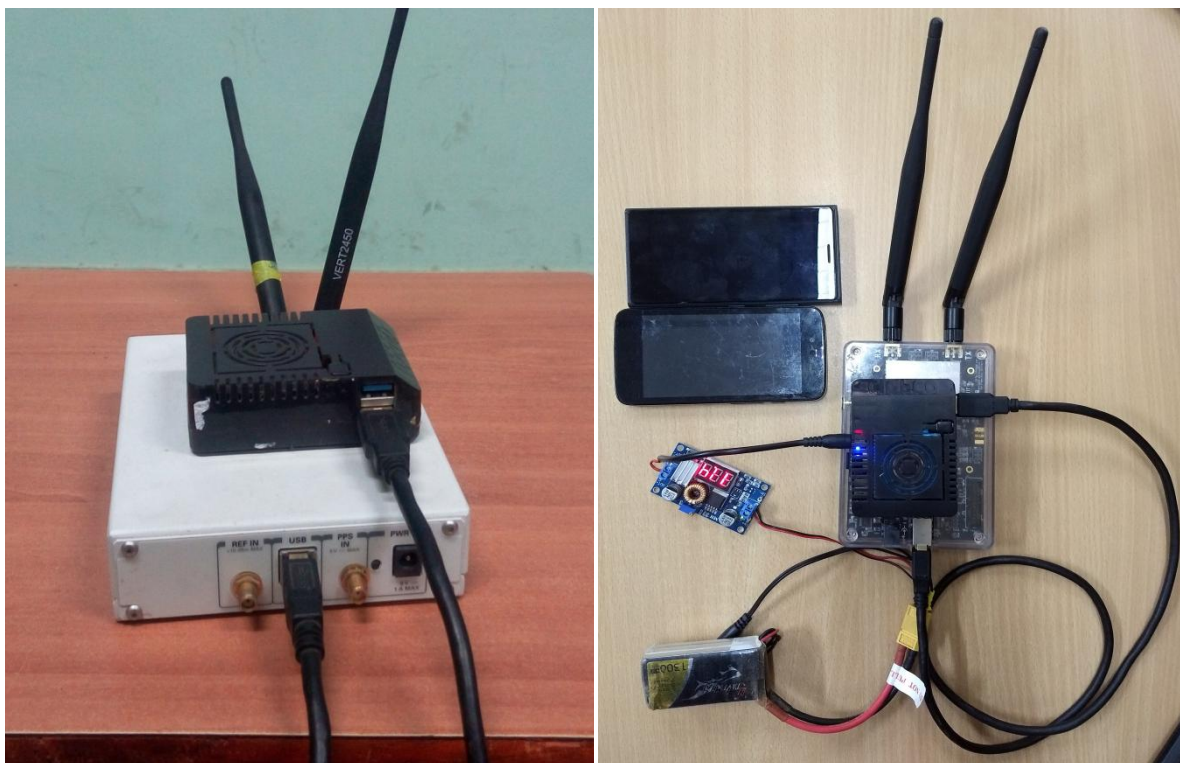
Fig 7.11: Network setup using Odroid XU4 with USRP B210 and BladeRF X40
