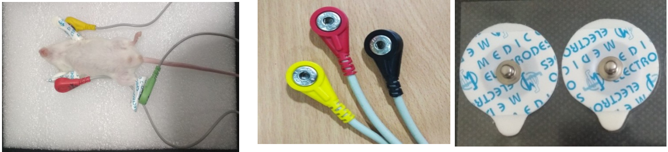
Figure 25: Electrodes placed on the paws of the mice to test the electrodes-skin interface and the electrolyte containing pads and electrodes
