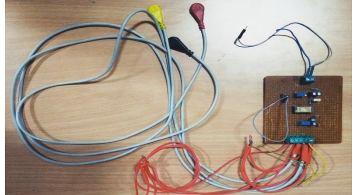
Figure 8: IC AD624 on board and whole ECG circuit with electrodes
