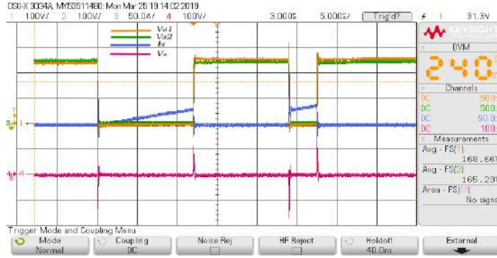
(a) Double Pulse waveform, C_s=11\text{nF} , R_g=14.7\Omega Scale; time: 5\mu\text{s}/\text{div} , device voltage: 100\text{V}/\text{div} , current: 50\text{A}/\text{div} , snubber voltage: 100\text{V}/\text{div}
