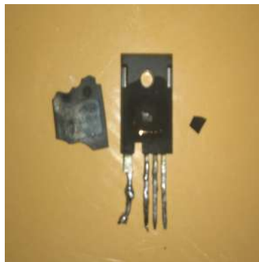
Figure 2.3: Photograph of failed SiC MOSFET
