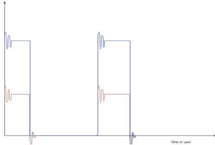
Figure 3.2: Individual device voltage in series connection without snubber circuit
