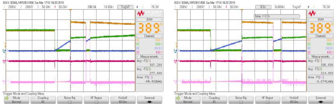
(a) Double Pulse 1. Scale; time: 10μs/div, voltage: 200V/div, current: 50A/div, snubber voltage:100V/div (b) Double Pulse 2 Scale; time: 5μs/div, voltage: 200V/div, current: 50A/div, snubber voltage:100V/div
