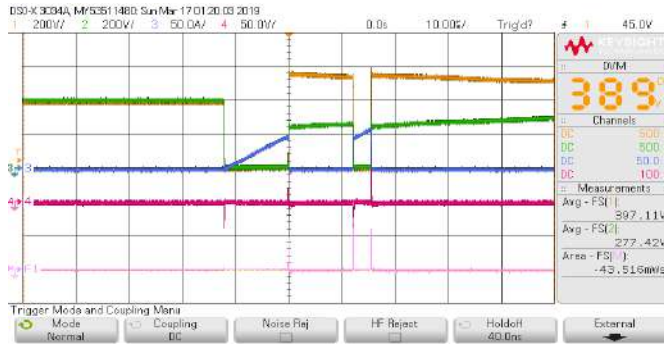
(c) Double Pulse 3 Scale; time: 10μs/div, voltage: 200V/div, current: 50A/div, snubber voltage:100V/div
