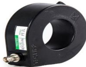
Fig 2.6: Basic HFCT Apparatus used in current Signal measurement
