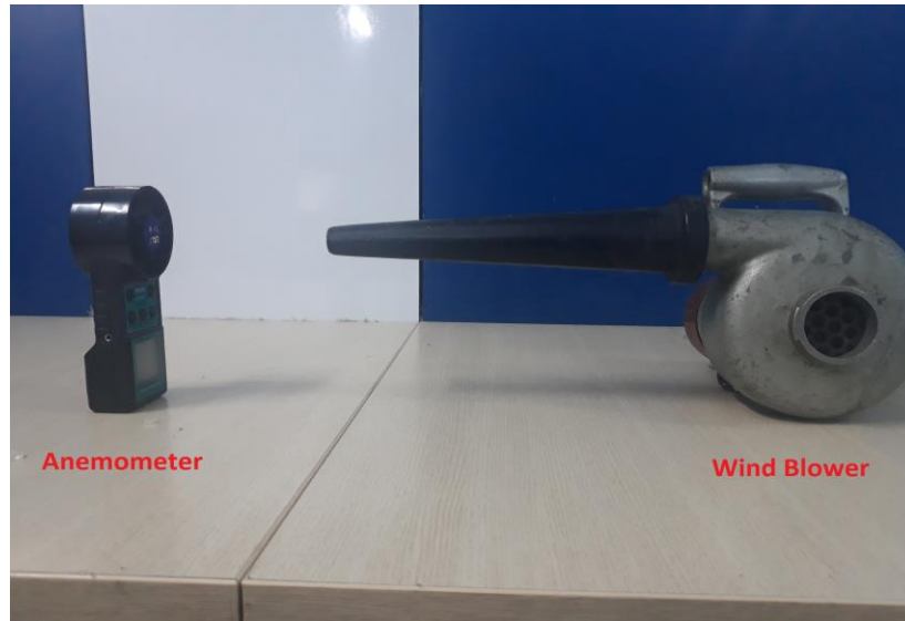
Figure 4.2: Wind speed measurement setup using anemometer
