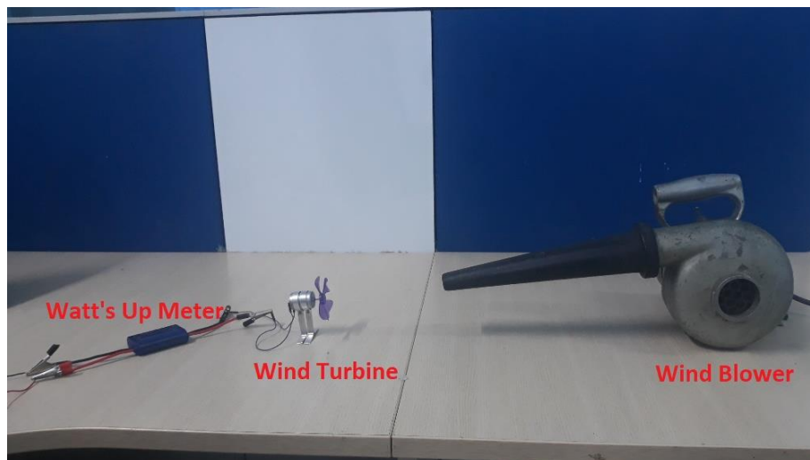
Figure 4.3: Energy generation using micro wind turbine and wind blower
