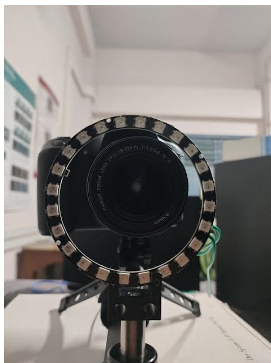
Figure 4.4: Ring of 24 LEDs around the camera
