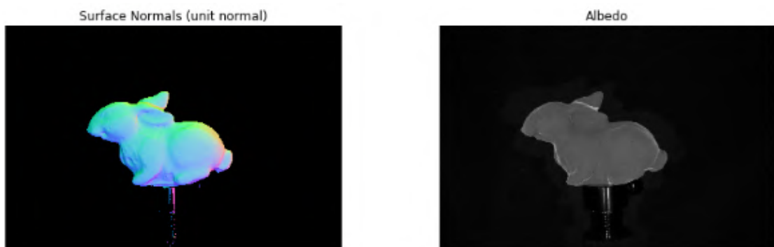
Figure 4.10: Photometric Stereo results on using only 3 images
