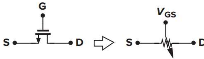
fig 5.3.1 MOSFET being used as variable resistor.
