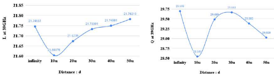
fig 6.3.2 c: Inductance and Quality factor simulated at 39GHz
