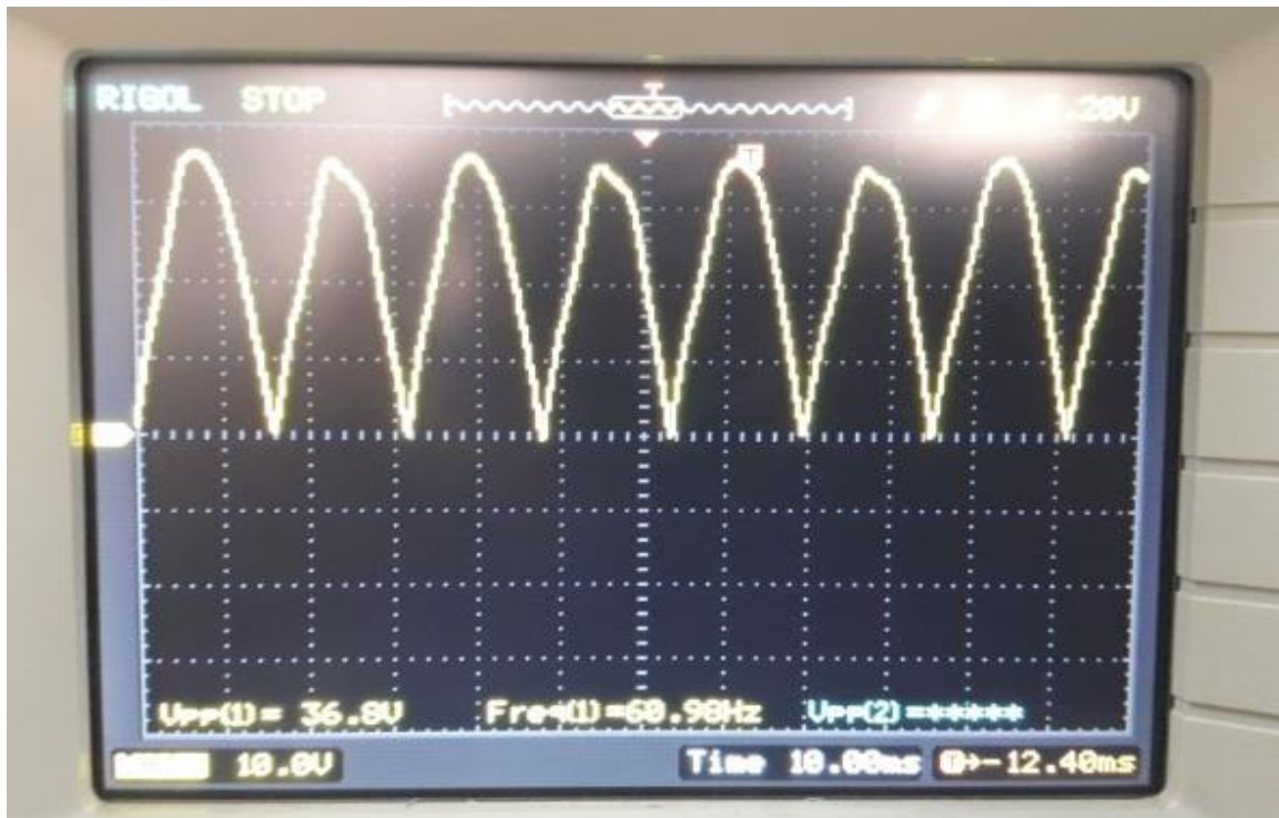
Fig. 2.7: Photograph of Half wave rectified output from Mide piezo strip on Digital Oscilloscope
