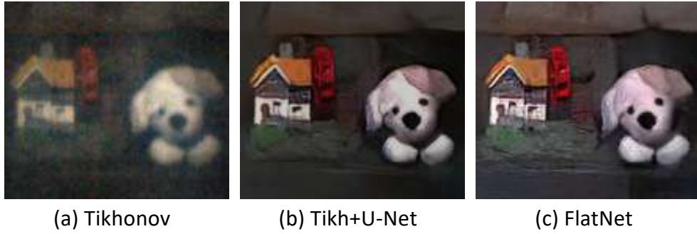
Figure 5.7: Comparison of FlatNet with Tikh+U-Net. Top row shows the comparison of FlatNet-sep with Tikh+U-Net while the bottom row shows the comparison of FlatNet-gen with Tikh+U-Net. FlatNet provides sharper and more photorealistic reconstructions compared to Tikh+U-Net for both separable and non-separable models.
