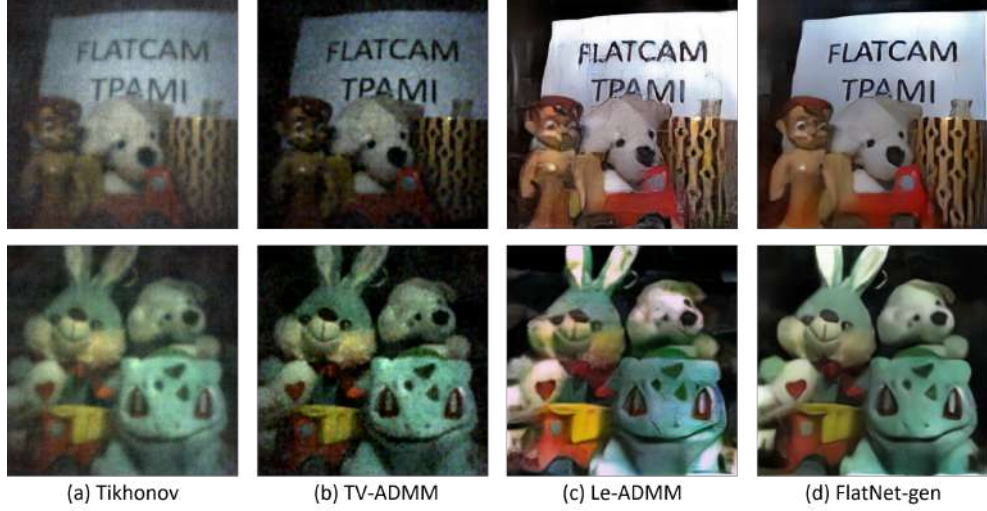
Figure 5.6: Direct Captured Reconstructions for PhlatCam. FlatNet-gen has fewer artifacts while Le-ADMM suffers from blurry reconstructions and hallucinated artifacts.
