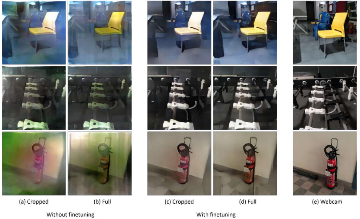
Figure 5.15: Cropped measurements for Unconstrained Indoor Scenes. We can observe that FlatNet-gen finetuned on unconstrained scenes provides reasonable reconstruction quality even for cropped measurements
