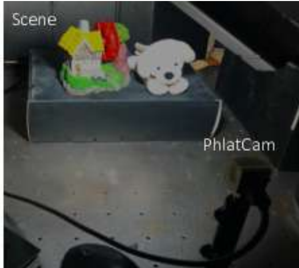
Figure 5.3: Direct Capture Setup. We collect measurements in a dark room, with the only source of illumination being a controllable light source. These measurements are more similar in distribution to monitor acquired images (display capture). Indoor measurements in the wild can however differ significantly from this.
