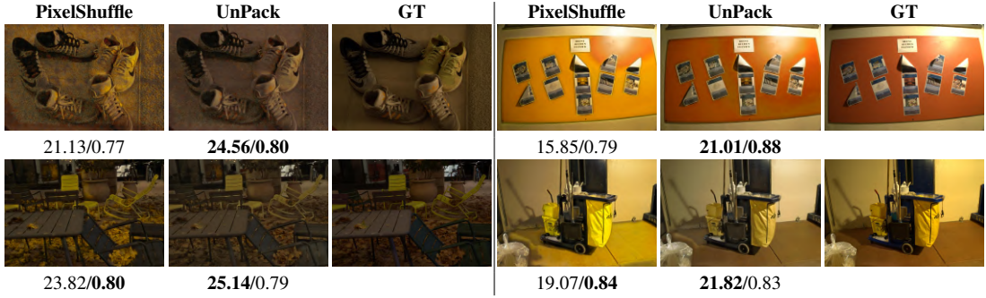
Figure 4.3: Comparison between the two upsampling methods with LLPackNet – PixelShuffle and UnPack, evaluated on the SID dataset. The UnPack operation helps to achieve better color restoration by reducing color distortions.
