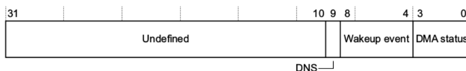
Figure 3.1: DMA Status Register bit assignments
