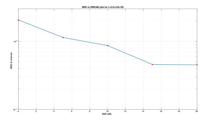
Figure 6.1: MSE of channel vs SNR (dB)
