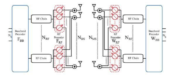
Figure 3.1: Block Diagram of BS-MS transceiver
