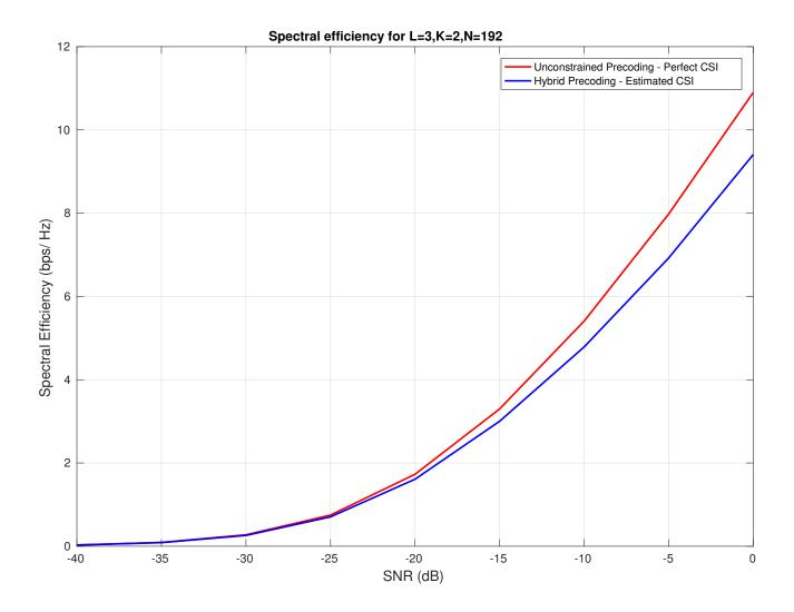
Figure 6.4: Spectral efficiency of the channel for  $L_d=3,\widetilde{K}=2$
