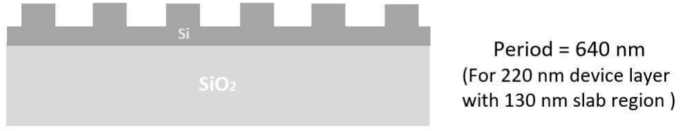
Figure 3.11: Grating coupler in 220 nm SOI : Side view
