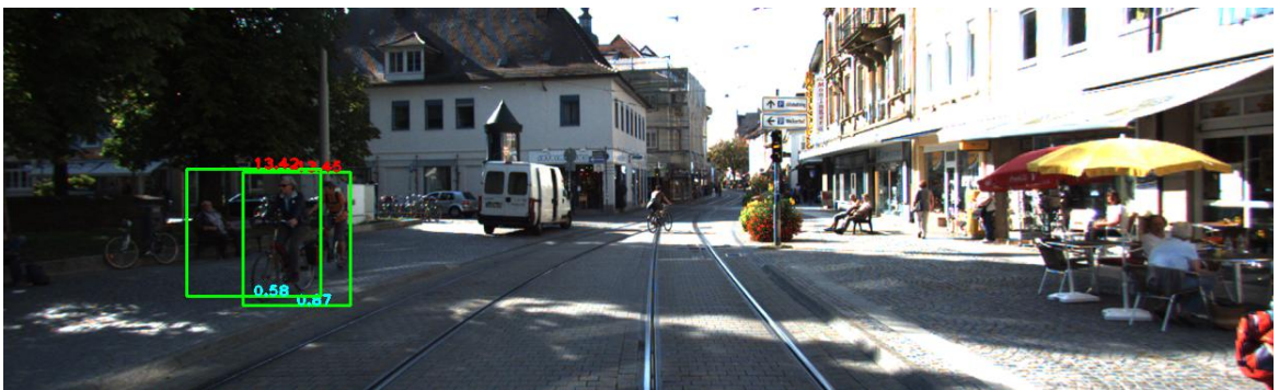
Figure 5.39: ZF based model: The detection took 0.0150 seconds in Nvidia Titan X GPU
