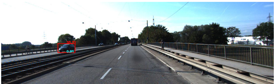
Figure 5.26: VGG based model: The detection took 0.0172 seconds in Nvidia Titan X GPU
