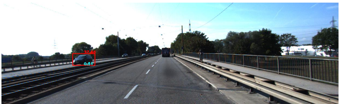
Figure 5.27: ZF based model: The detection took 0.0153 seconds in Nvidia Titan X GPU
