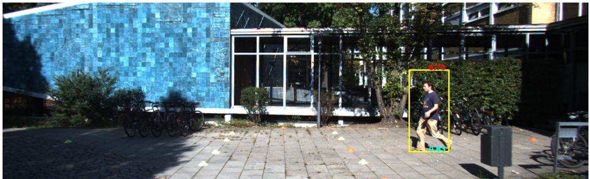
Figure 5.29: VGG based model: The detection took 0.0168 seconds in Nvidia Titan X GPU
