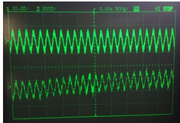
Figure 3.4: 1kHz signal at the top and signal captured from the TMR sensor at the bottom
