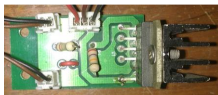
Figure 3.2: OPA 541 power amplifier circuit board used to provide current to the wire
