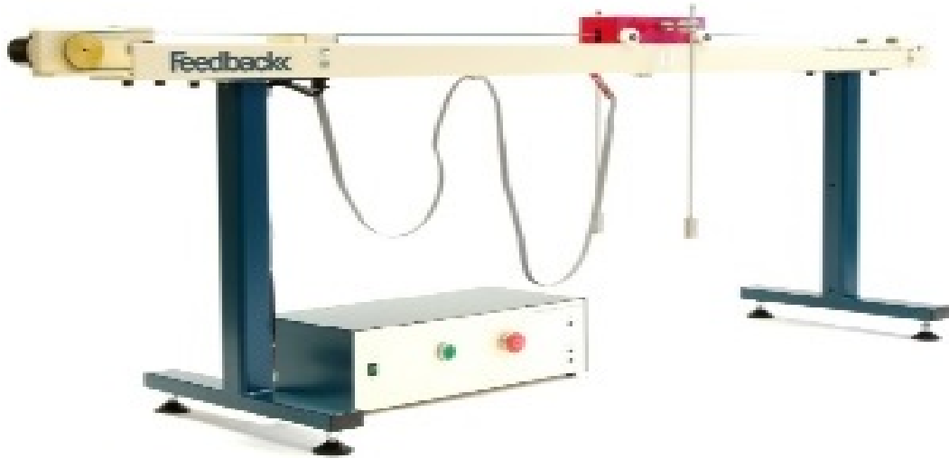
Figure 2.1: Pendulum on a Cart setup used for experiments[3]
