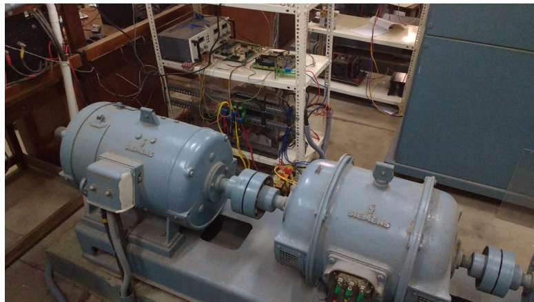
Figure 3.1: Machine setup for implementing the field weakening strategy
