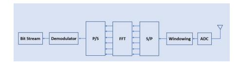
N samples are windowed from N+Ncp received samples, these set of N samples are passed through the FFT stage. The receiver processing in AW-OFDM is very similar to that of OFDM.
