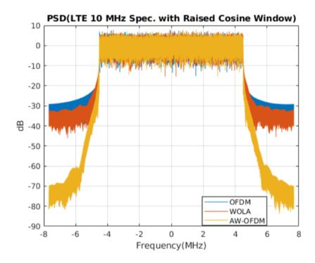
This show that AW-OFDM has a very high side-lobe suppression compared to OFDM and WOLA-OFDM, which is a great advantage for any waveform because the guard bands needed for the side-lobe suppression becomes very less. Hence AW-OFDM can transmit more data in a given band compared to OFDM and WOLA OFDM, in other words this waveform provides high spectal Efficiency.
