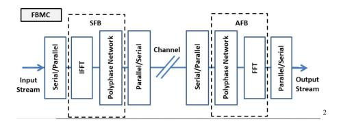
From the above mentioned figure it shows that the transmitter and the receiver use polyphase Network which is a filterbank introduced to reduce the sidelobe leakage. When carriers were modulated in an OFDM system, sidelobes spread out either side. With a filter bank system, the filters are used to remove these and therefore a much cleaner carrier results.
