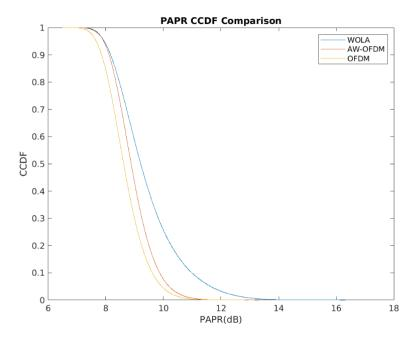
Increaded PAPR at the transmitter leads to saturation in the Power amplifier stage, which leads to loss of orthogonality at the subcarrier levels. This result shows that the PAPR of AW-OFDM is smaller compared to WOLA-OFDM and its comparable with that of OFDM.
