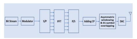
Symbols are modulated using IFFT and added with Cyclic prefix. After the cyclic prefix is added and an asymmetric window operation is done with a sample overlap. This is transmitted through the channel. The transmitted samples are N+Ncp samples per block, hence have the same overhead/spectral efficiency as OFDM.
