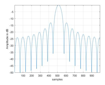
It is very clear from the response of the digital sinc that its response reduces down very slowly, the second sidelobe is 13dB slow than than the main lobe. This property of the digital sinc causes huge out of band leakage for OFDM in the frequency domain.
