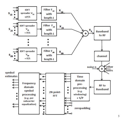
In the above figure UFMC use B number of filters during the transmission to reduce the Power leakage. UFMC provides lower sidelobe leakage compared to OFDM but higher leakage compared to FBMC.
