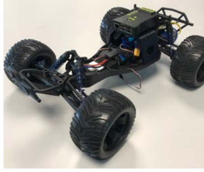
Figure 7.12: Erle Rover used for data logging
