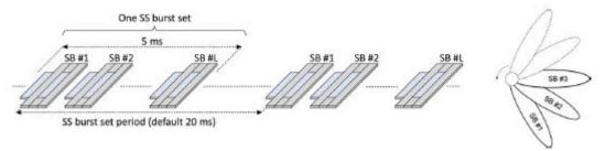
So, each SSB's periodicity is period of SSBurst set. Using 64 SSBs' for high frequency usage can be justified as using large number of SSBs' in one SSBurst takes more slots so more time in lower frequency range but with high frequency usage ,we use larger SCS, taking even less time per NR slot.
