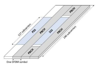
**B**efore going into structure of SSB, Physical Cell ID (PCI) is determined by two components  $N_{ID}^{(1)}$  and  $N_{ID}^{(2)}$ . 5G NR provides us with 1008 unique cell IDs. And ID-1 is contained by SSS and ID-2 is contained by PSS.
