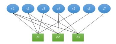
If data and parity bits are represented by  $c_i$  {i=1, 2, 3, 4} and {i=5, 6, 7} respectively, error bits represented by  $e_i$  then the above graph can be interpreted in terms of equations given below:
