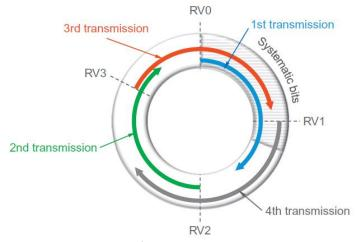
Final step in rate-matching is interleaving of bits.
