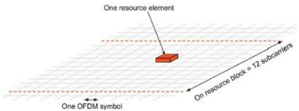
If SCS = n \* 15KHz then NR slot period  $= 1/2^{n-1} ms$ . For example, if n = 2 then NR slot period for 30KHz SCS is 0.5ms
