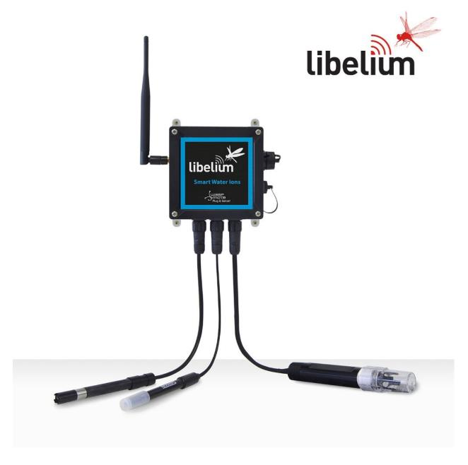
This device is capable of taking all the readings required and upload the data using cellular or long range zigbee protocol to the cloud. This is a low power device usually used in chemical detection and pollution level. It could sustain years with their battery. The only major drawback is that they are very costly and are typically used to monitor the properties at a certain location.
