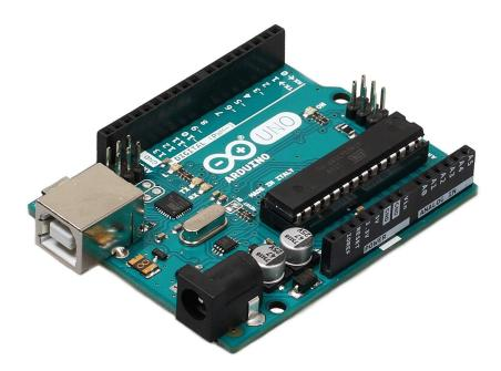
Arduino uno, the variant used in this project has ATMEGA328P as its microprocessor. It is capable of supporting 14 digital I/O and 6 Analog input pins. It also has a USB port to program
