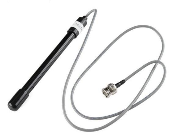
It supports 3~5v wide voltage input, and is compatible with 5V and 3.3V main control board; The output signal filtered by hardware has low jitters; The excitation source adopts AC signal, which effectively reduces the polarization effect, improves the precision and prolongs the life of the probe; The software library uses two-point calibration method, and can automatically identify
