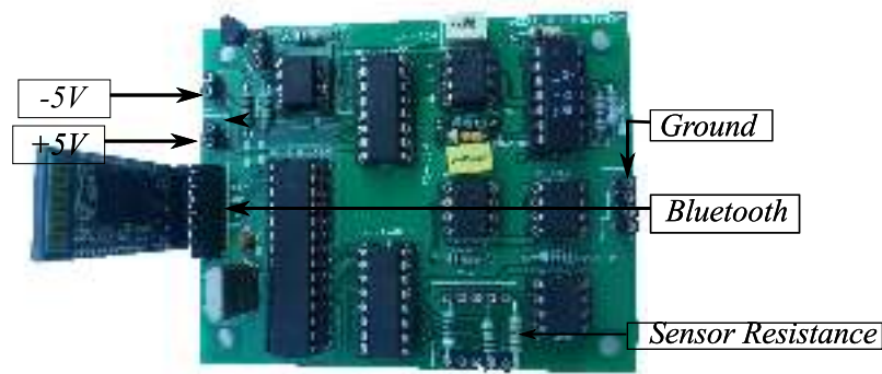
Fig. 4.7 Components mounted on double layer PCB
