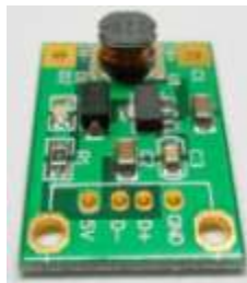
Figure 5.4: DC-DC Boost Converter Step Up Module 1-5V to 5V 500mA [11]
