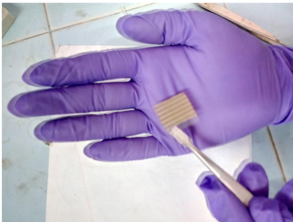
Fig. 3.8 Solar cell after metallisation (Al metal)
