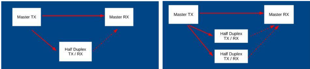
Fig 4.2: Configurations for (a) a conditional relay, and (b) two conditional relays
