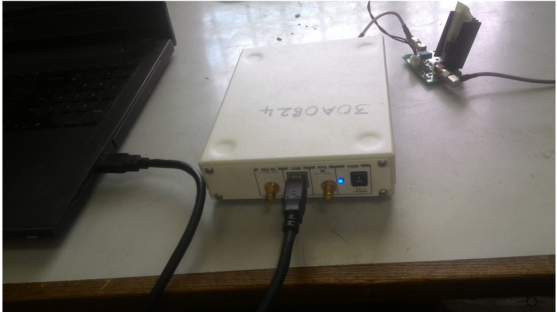
Figure 6.2: A picture of the setup with USRP 2901 and power amplifier (PCB 1)
