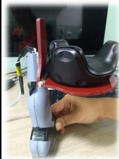
Figure 7 - The Vive tracker attached to an ultrasound probe (dummy).
