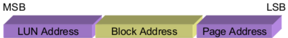
Figure 3.7: Row address layout[5].
