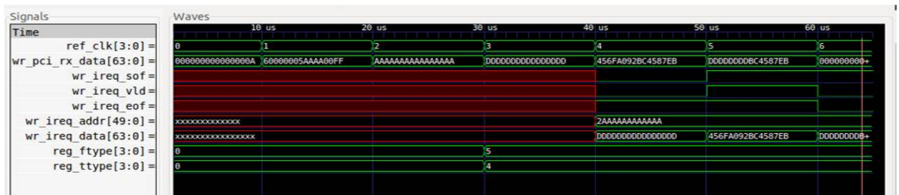
Figure 5.6: Simulation Result of Test case- MemWr 64 Bit Address 5DW Data
