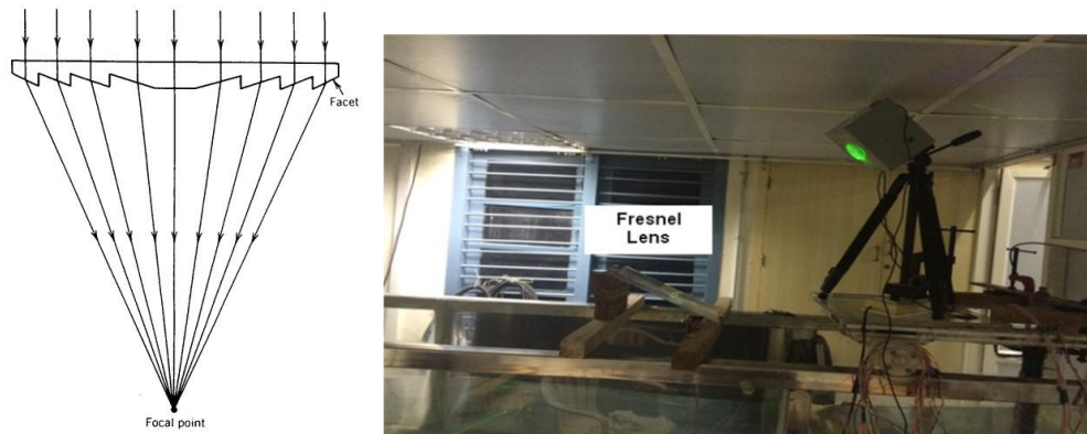
Figure 4.9: Use of Fresnel lens to increase receiver aperture
