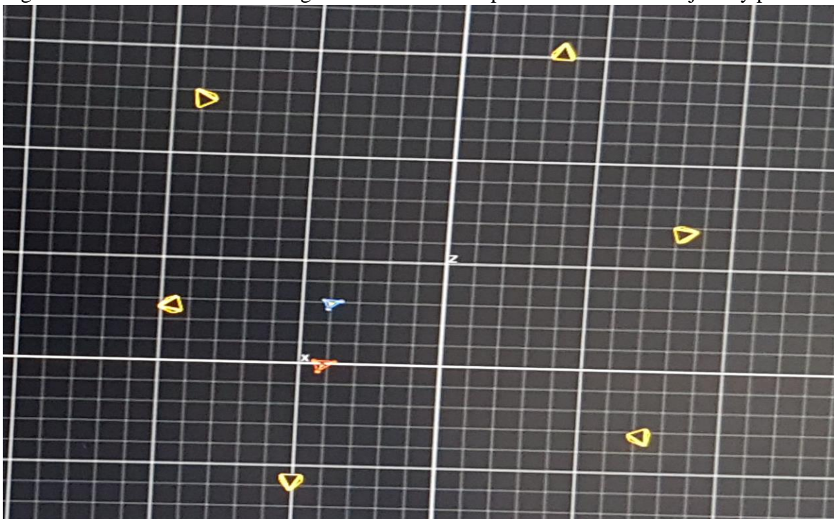
Figure 13: Picture Depicting the Opti-Track system in the Lab. The Blue rigid body is the pursuer. The Red rigid body is the evader. The Yellow Markers represent the cameras of the Opti-Track system
