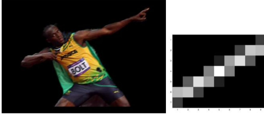
Figure 2.4: Synthetically blurred input with associated ground truth kernel
