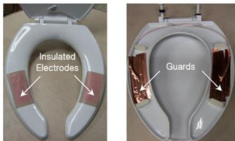
Fig. 2.5 capacitive ECG in the toilet seat [3]
