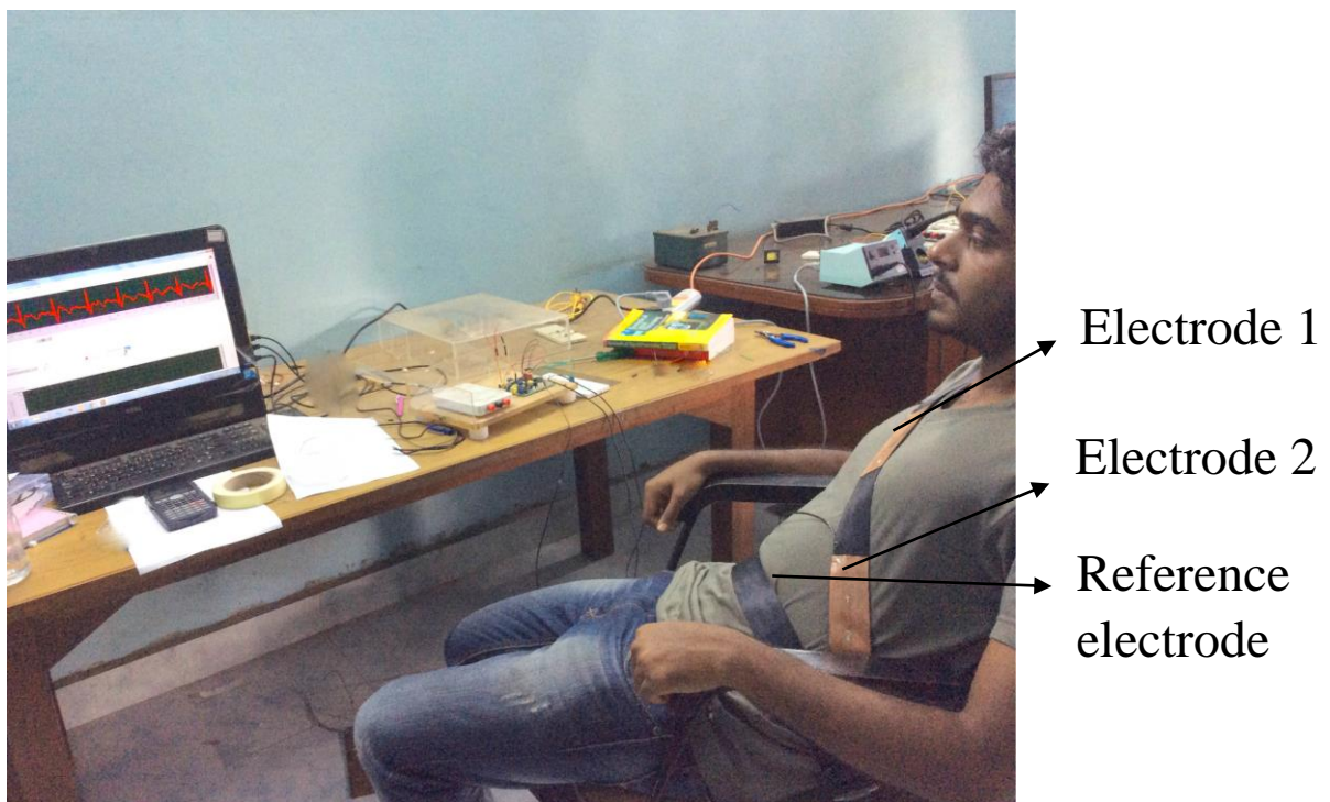
Fig 4.9 shows a subject wearing a single layered shirt (T-shirt) whose ECG is being recorded
