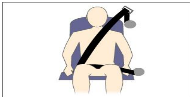
Fig 4.1 A typical 3-point BIS configuration
