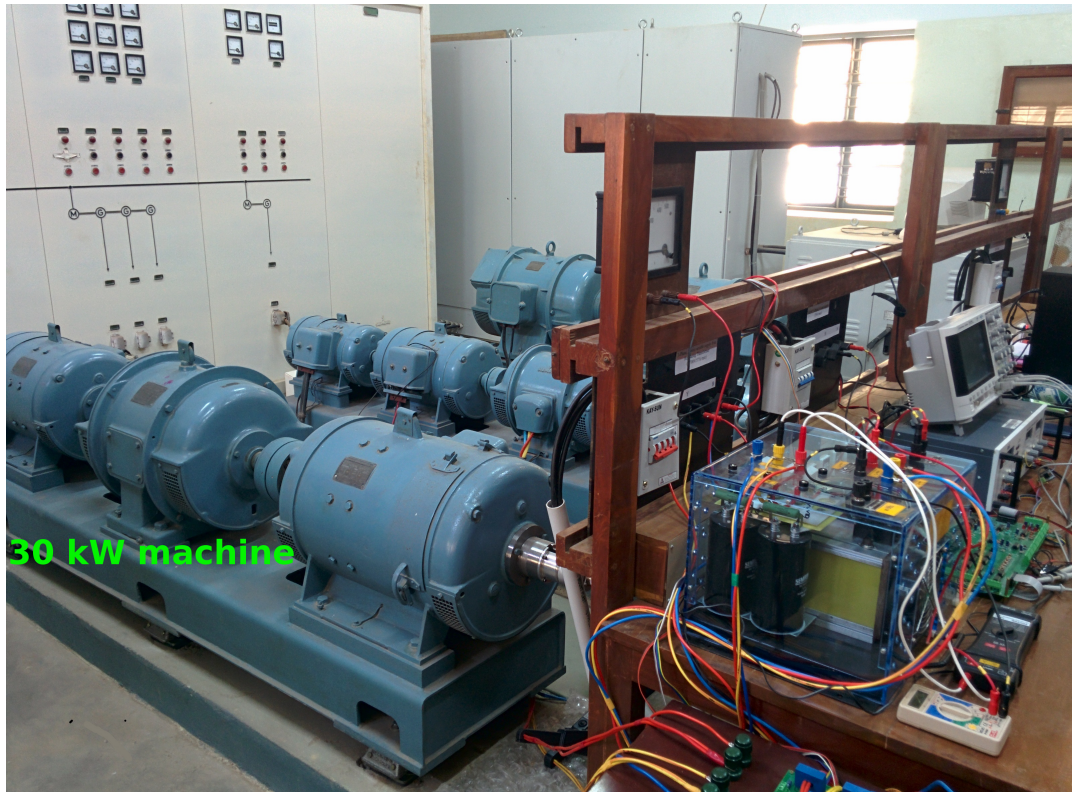
Figure 3.9: Machine setup for implementing vector control
