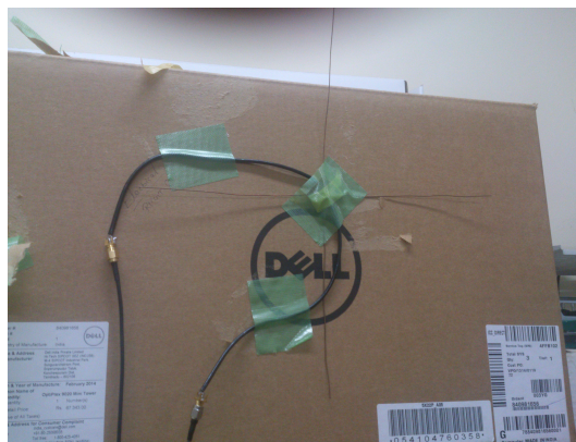
Figure 3.3: Hand made hybrid antenna
