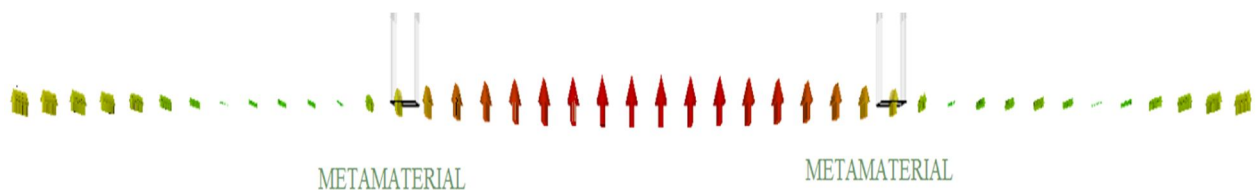
Figure 4.8: Electric field propagation through the metamaterial indicates constant phase inside the medium as the field arrows are not flipped upon many distances.
