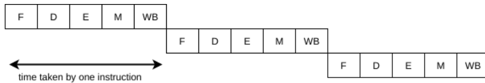
Figure 2.2: Instruction processing in single cycle machine
