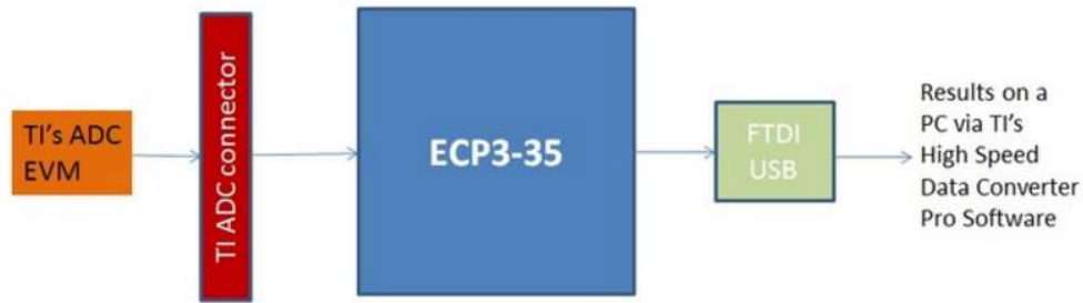
Figure 2.5: Functional block diagram of TSW1405 5
