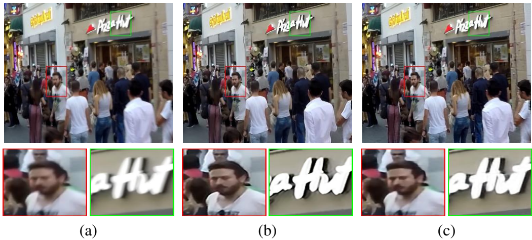
Figure 5.3: Comparison with Sun et al. (2015). (a) Space variantly blurred input image. (b) Deblurred output of Sun et al. (2015). (c) Output of our network.
