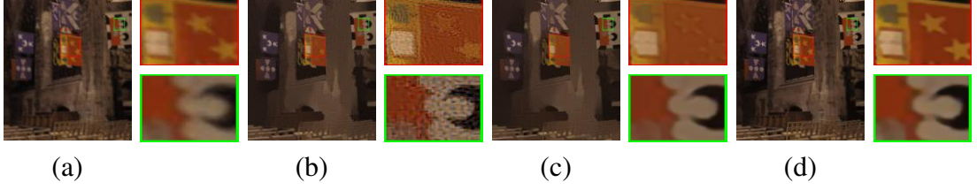
Figure 1.1: Effect of image prior. (a) Input blurred image. (b-d) Deblurred result using Pan et al. (2016) with (\lambda = 0.04, \mu = 0.007, \lambda_{TV} = 0.001) , (\lambda = 0.001, \mu = 0.01, \lambda_{TV} = 0.01) and (\lambda = 0.004, \mu = 0.005, \lambda_{TV} = 0.01) , respectively.
