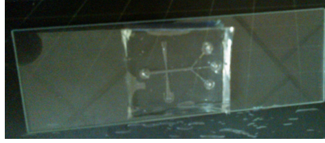
Figure 2.3: Molded PDMS device
