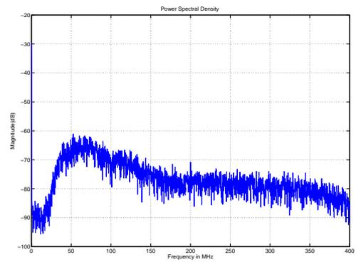
Figure 4.8:  $f_s = 800 \text{ MHz}$  , In-band noise =  $-67.01\text{dB}$
