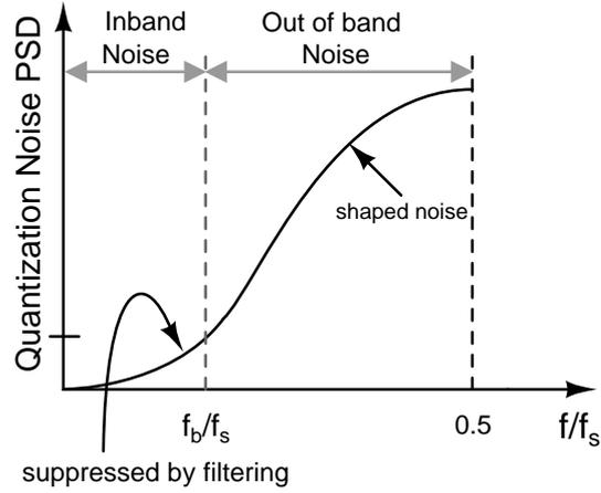
Figure 2.4: Spectrum of the shaped quantization noise.
