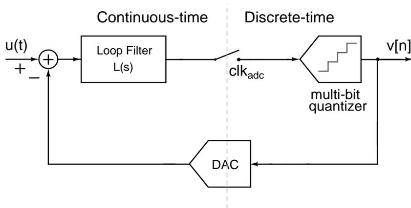
Figure 2.5: Block diagram of a continuous-time modulator.[3]
