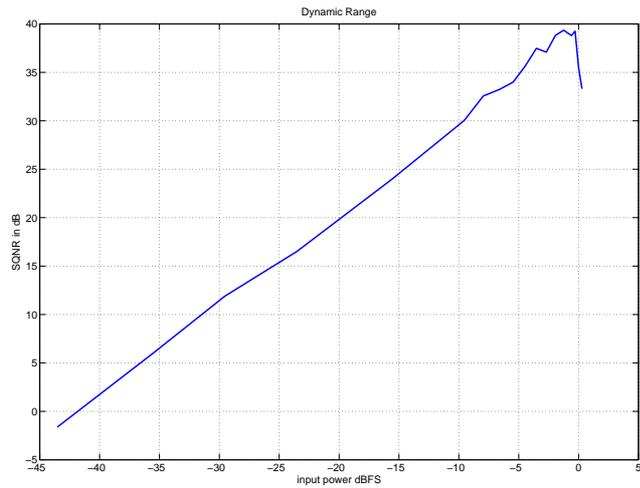
Figure 4.11: SQNR vs input amplitude for OSR= 25 and input of 5MHz
