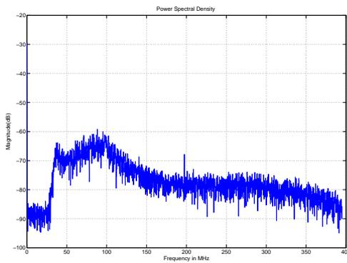
Figure 4.7:  $f_s = 790 \text{ MHz}$  , In-band noise =  $-67.08\text{dB}$
