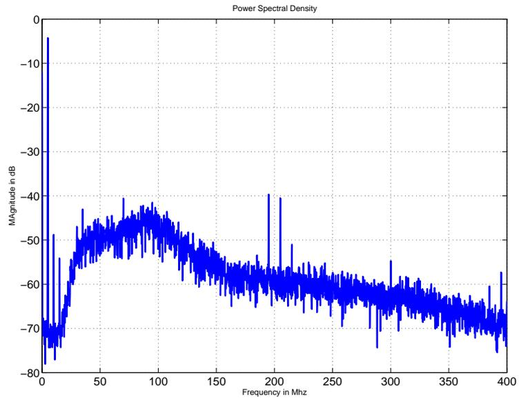
Figure 4.9: Output PSD for OSR of 25 and input of 5 MHz
