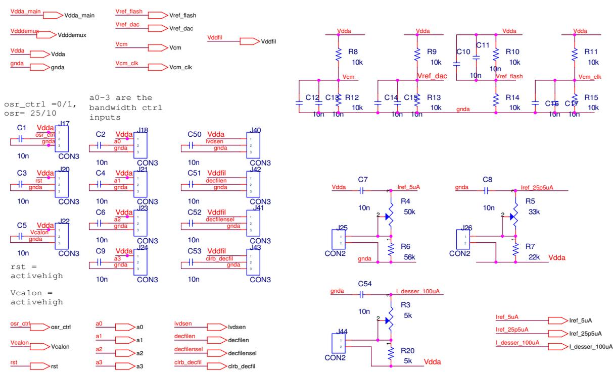
Adjust bias currents by measuring the dc voltages across the connectors. Measure the resistance accurately. Disconnect the multimeter while measuring the DSM.
