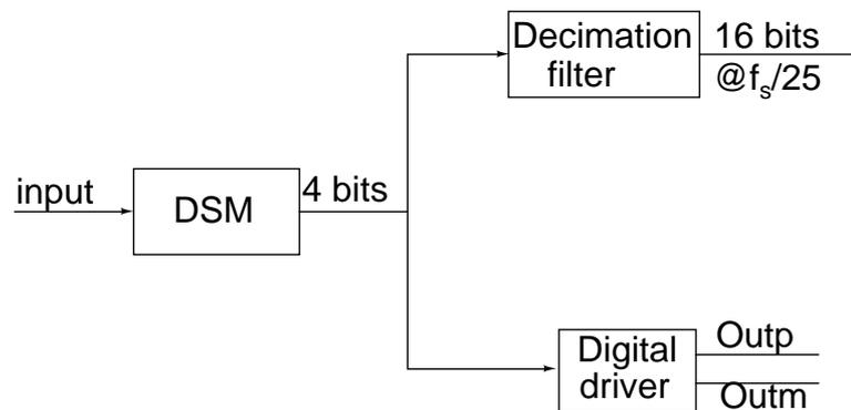
Figure 3.1: Block diagram of ADC
