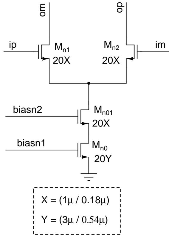
Figure 3.2: Schematic of unit DAC cell[1]
