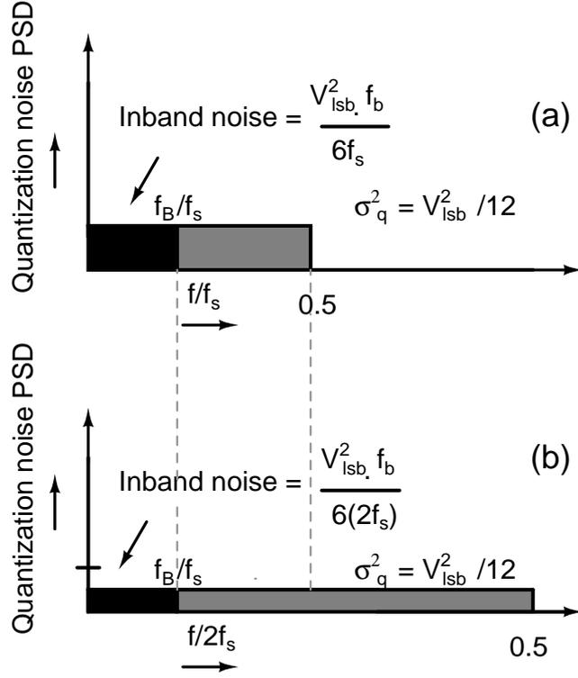
Figure 2.2: Quantization noise spectrum of ADC. (a) Sampling at  $f_s$  (b) Sampling at  $2f_s$ . [3]
