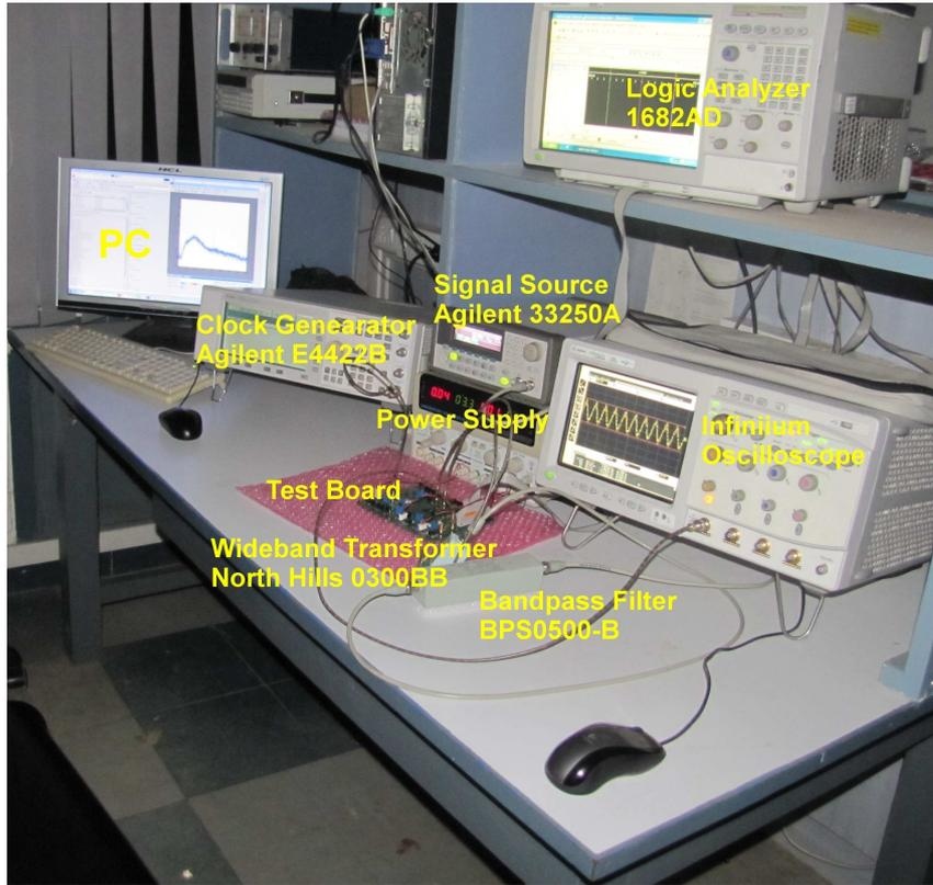
Figure 4.4: Snapshot of test setup
