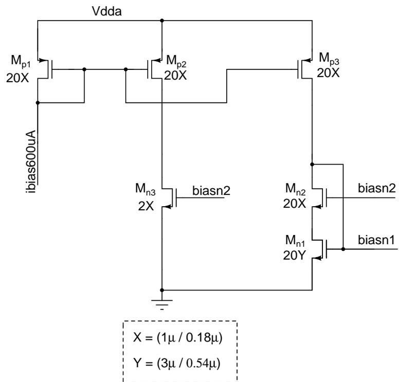
Figure 3.3: Bias generation circuit for DAC cells[1]
