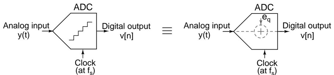
Figure 2.1: (a) ADC (b) Additive quantization noise model.[3]
