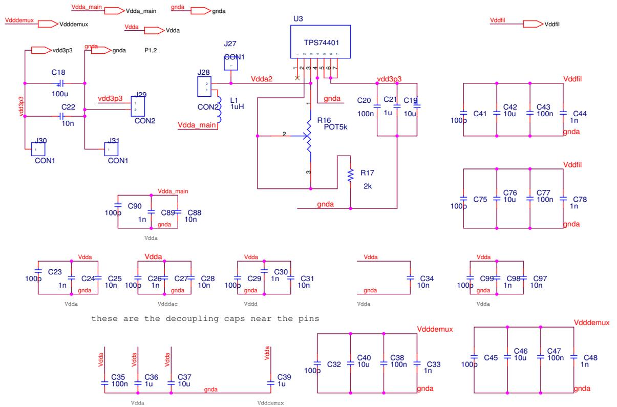
TPS74401 is a low dropout linear regulator capable of supplying 3A at 3.3 V (max).
