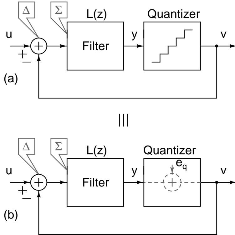
Figure 2.3:  $\Delta \Sigma$  modulator.[3]
