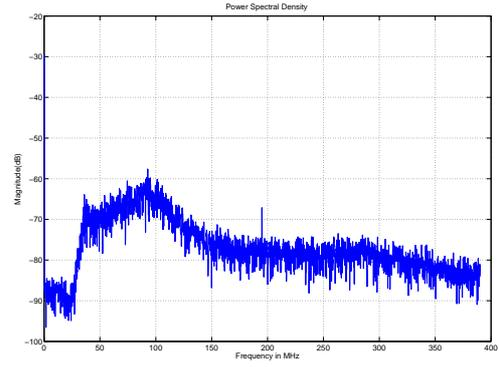
Figure 4.6:  $f_s = 780 \text{ MHz}$  , In-band noise =  $-67.45\text{dB}$
