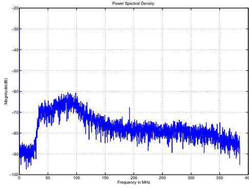
Figure 4.5:  $f_s = 770 \text{ MHz}$  , In-band noise =  $-67.55\text{dB}$
