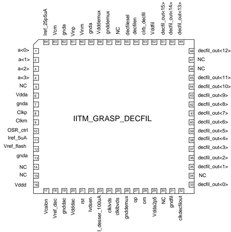
Figure 4.1: Pin details of the chip
