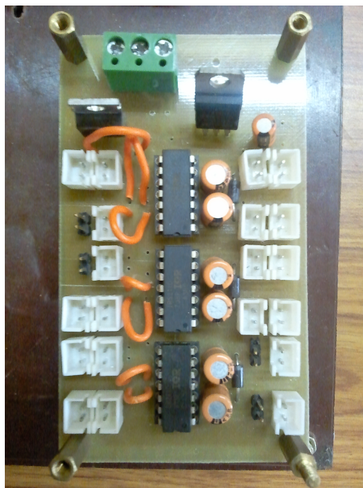
Figure 3.7: Gate drive circuit for inverter
