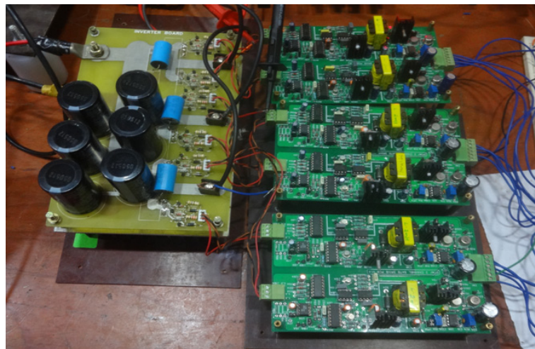
Figure 4.2 Hardware implementation of three phase 1 KVA inverter
