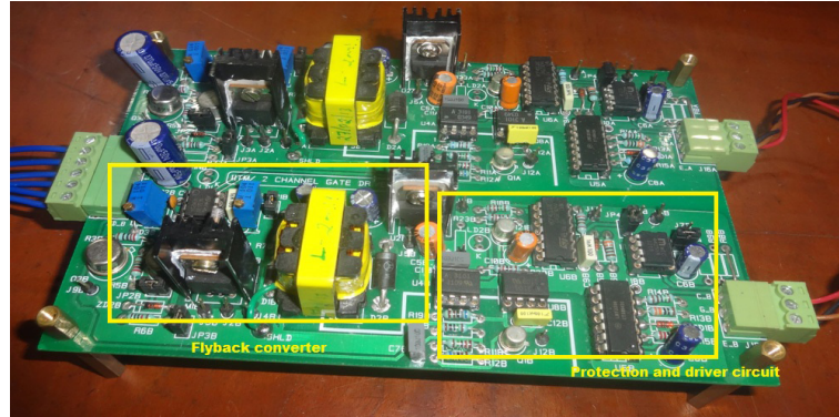
Figure 2.12 Hardware implementation of gate drive circuit
