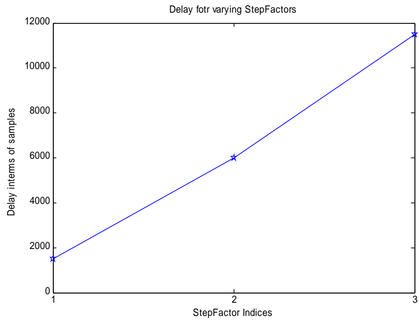
Figure 3.5: Convergence Delay with varying Step_factors at 0dB input power
